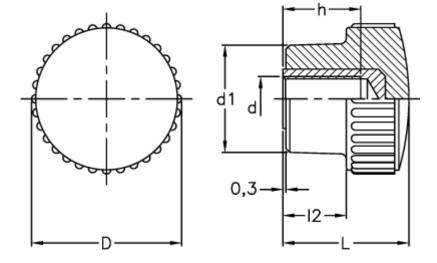
$$\begin{array}{ll} D & = 21 \\ d1 & = 13 \\ d \ 6H = M5 \\ h & = 16 \\ L & = 25 \\ I2 & = 12 \end{array}$$
